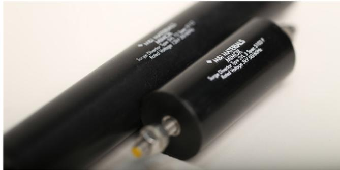
Each diverter consists of a number of metal oxide varistors, connected in series and encapsulated in a PVC container using a polyurethane resin. Dimensions of the diverters can be seen in Figure 1.
