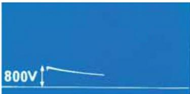
Figure 3 - With Metrosil (Type 300A/S1) Passing 10mA Connected Across the Coil
